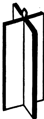
FIG. 135. TYPE OF PLUMB-BOB USED IN PLUMBING MERIDIAN DOWN A SHAFT.
